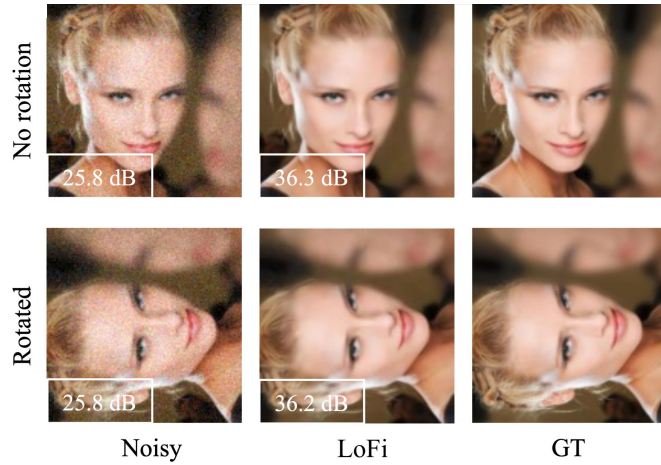
Fig. 16: Rotation equivariance analysis for LoFi architecture; LoFi exhibits minimal degradation in reconstruction quality when the input noisy image undergoes a 90-degree rotation.
